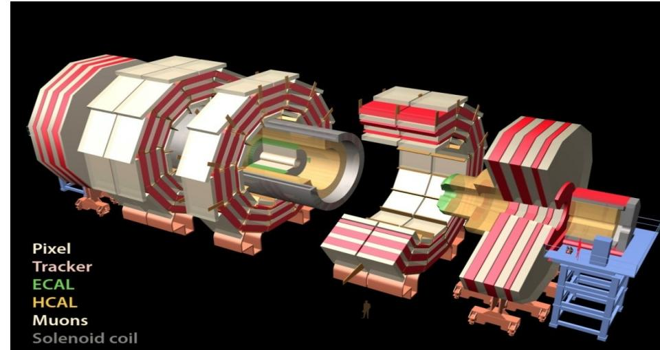
Total weight 12500 t, Overall diameter 15 m, Overall length 21.6 m, Magnetic field 4 Tesla
